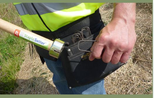
Pushes staples all the way into the ground NO moving parts
